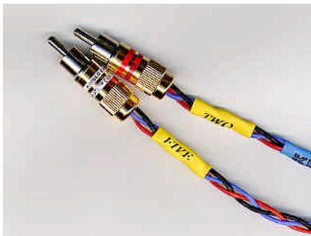
Each incoming interconnect was 1 meter in length, as was each outgoing interconnect, so the signal path consisted of one RCA - 1 meter of interconnect - one wiper contacting the resistor - 1 meter of interconnect - one RCA. The entire unit, when finished, only weighed a couple of pounds. The leads were not only numbered on the
